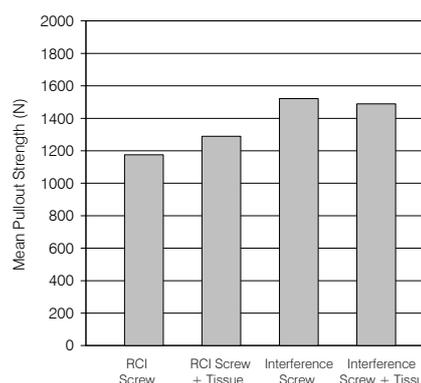
Figure 5 Post fatigue tibial fixation test results
